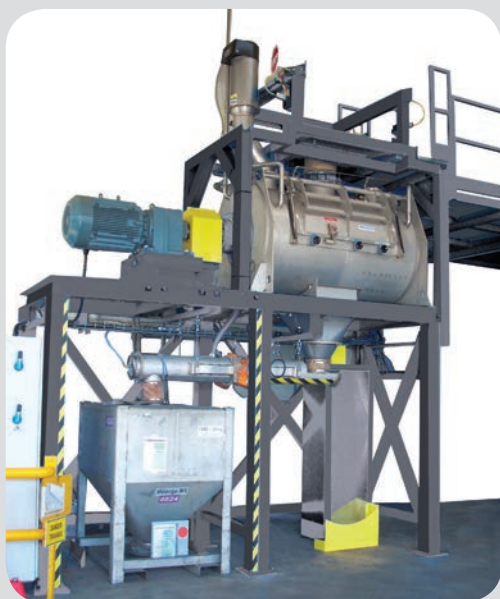
Mixing unit for metallic powders, in an inert atmosphere, and packaging in a flowbin.
