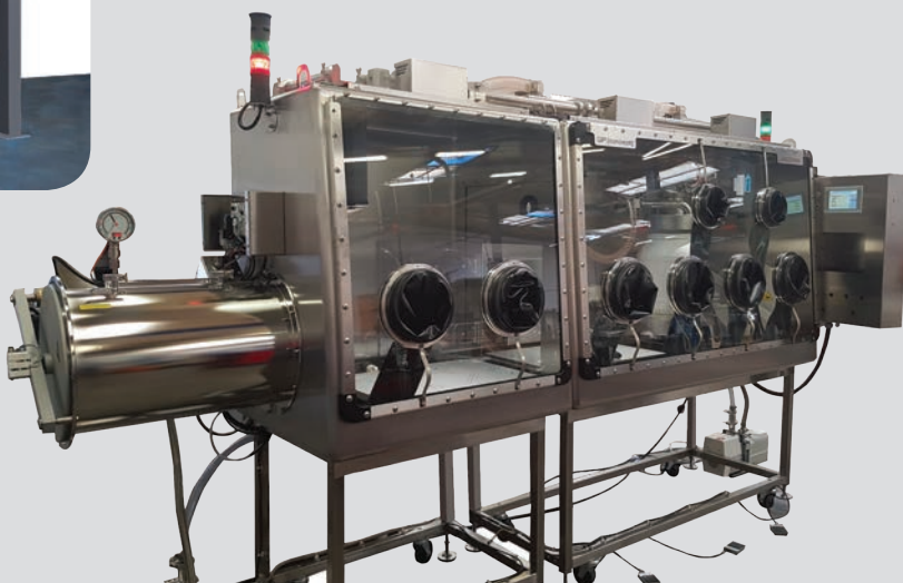
Very high contained dosing and packaging unit Use of Glove-boxes with controlled inert atmosphere.
